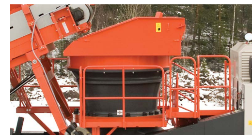
High performing CS440 Cone with ASRi
