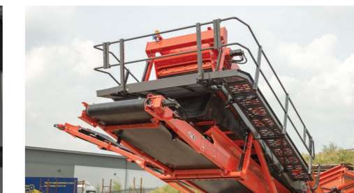
Three sided walkway around main conveyor
