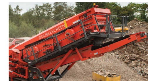
Hydraulically folding walkways for ease of maintenance
