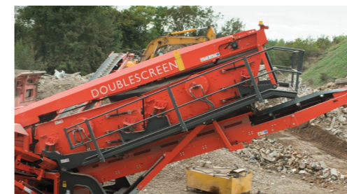
Patented triple deck Doublescreen technology
