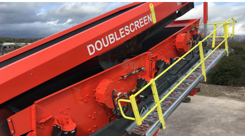
Hydraulically folding walkways for ease of maintenance
