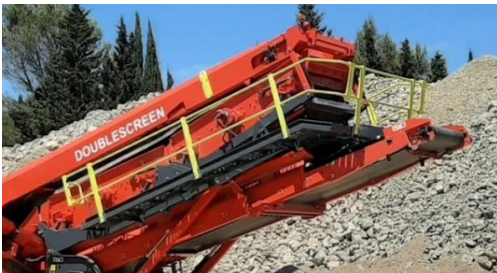
Two-deck Doublescreen with independent screen angle adjustment and screen separation
